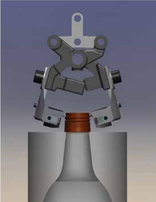
*Self adjusting POCO holder, with a thread pick-up GM insert, starts to close*
