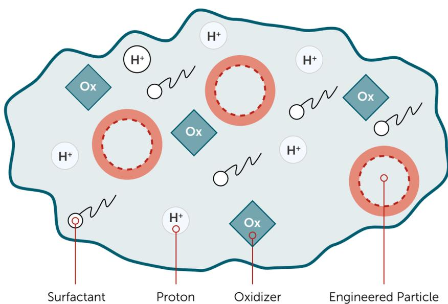
The purpose is to rapidly create and remove a nanoscale layer from the wafer surface with each pass.
