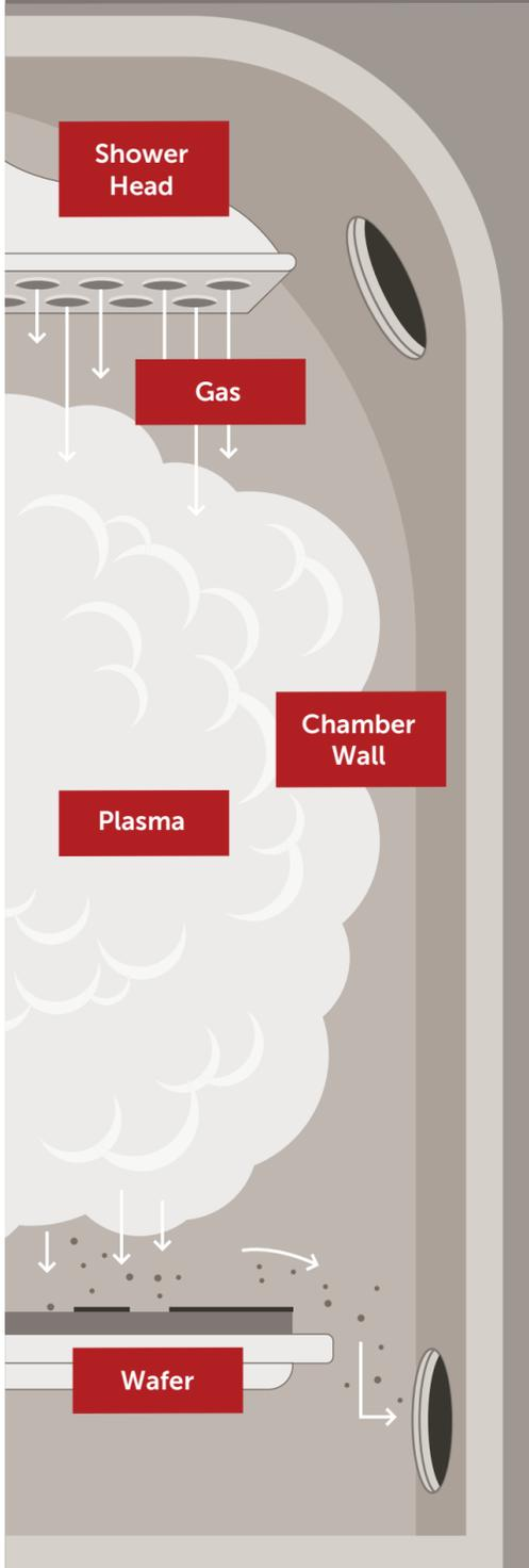
Traditionally, chamber parts and components in contact with wafers or chemicals were coated with metal oxides using plasma spray, anodization, and vacuum kinetic spraying.
