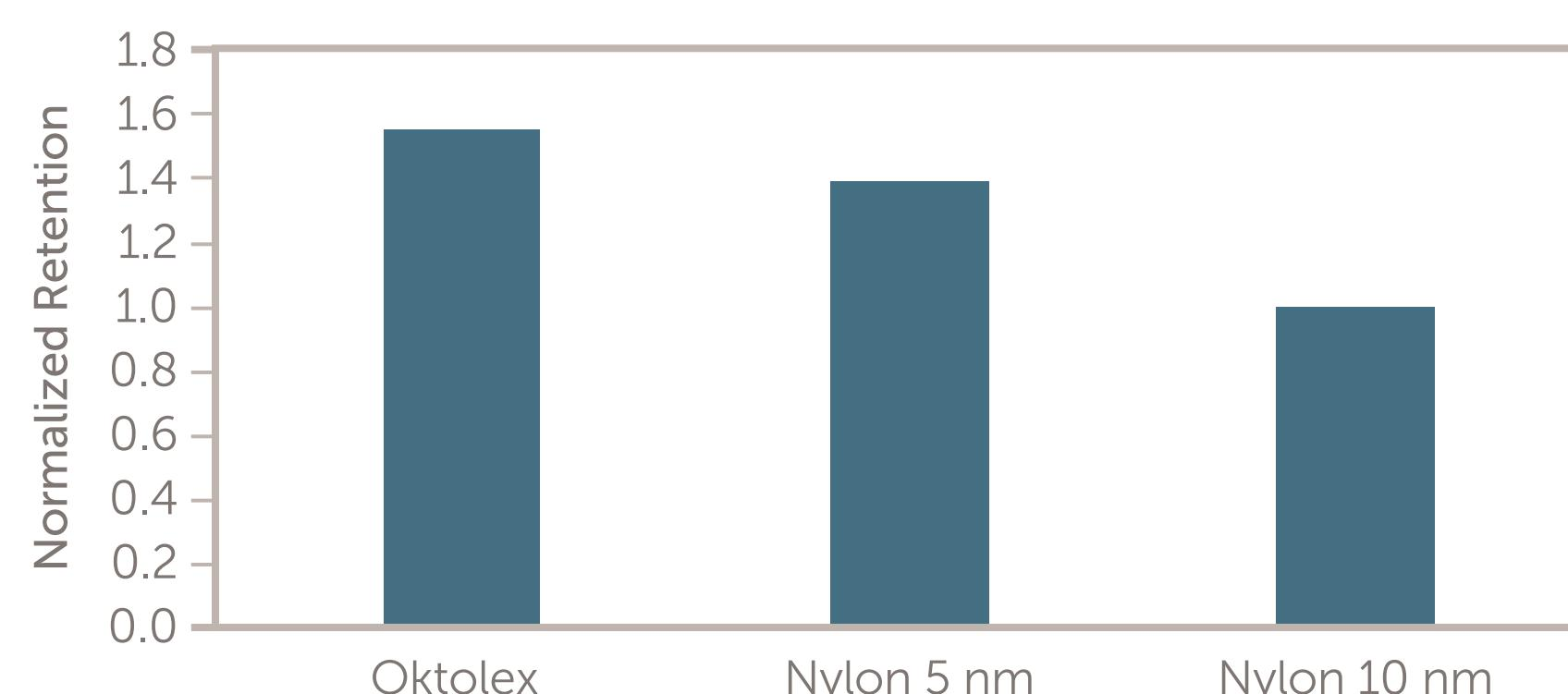
The Oktolex membrane has additional particle capture capabilities due to the membrane modification, making this membrane more retentive than either nylon membrane.
