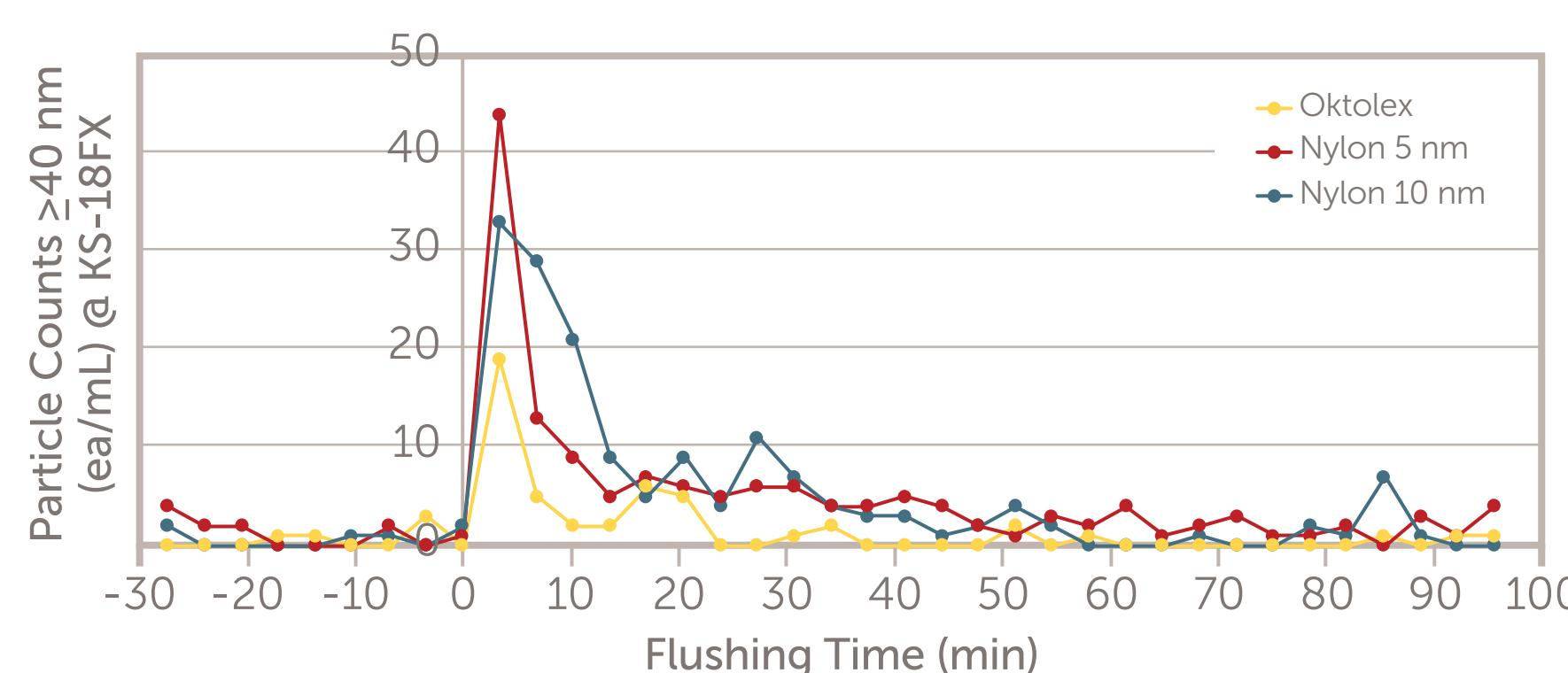
The Oktolex filter not only had the lowest level of particle counts at start-up, but also reached baseline more quickly than the comparison nylon filters.
