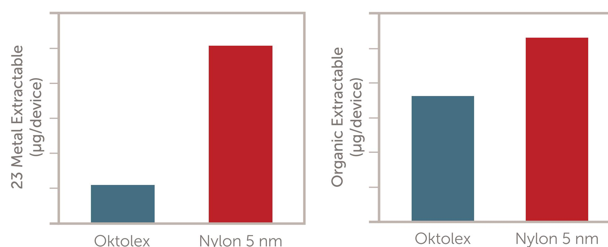
The Oktolex membrane showed lower extractables than the 5 nm nylon, suggesting that the nylon membrane released more undesirable contaminants into the solution, potentially leading to either long flush-up times to achieve baseline, or coating defects.
