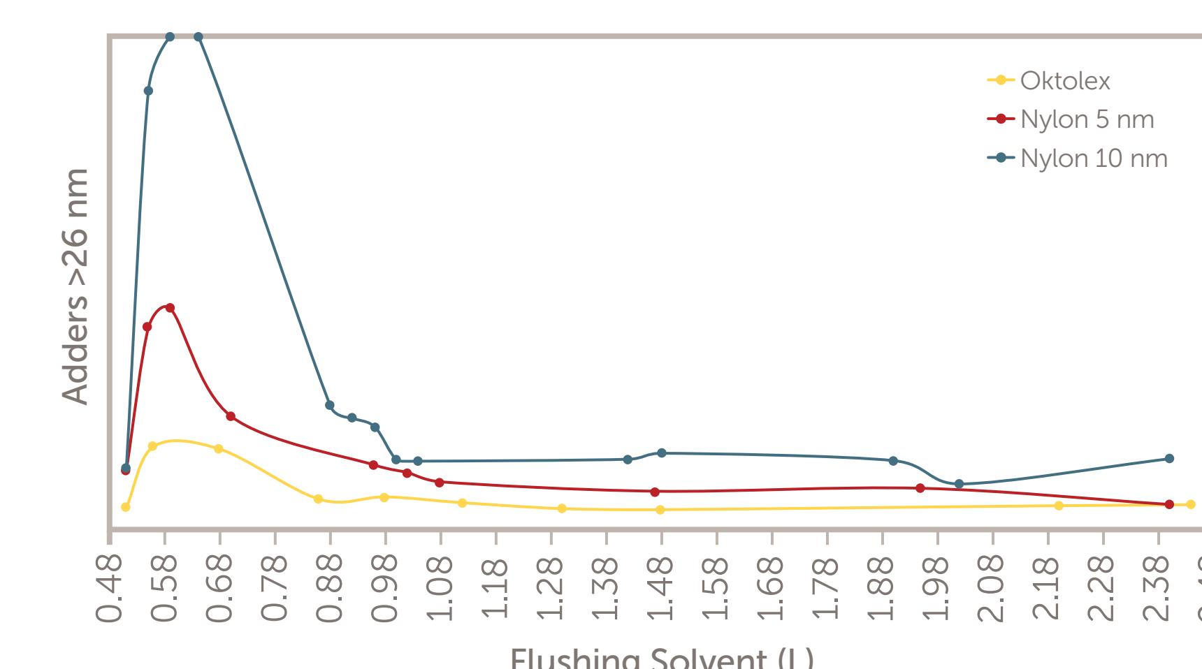
The Oktolex filter had a much lower number of 26 nm particles at startup, and reached baseline more quickly than the comparison point-of-use filters.
