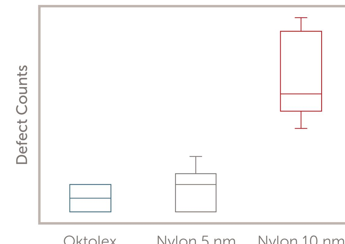
Further patterned defect studies on a 45 nm line, 100 nm pitch mask confirmed the performance of the Oktolex filter with significantly fewer single-bridge defects than the nylon filters.
