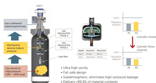
Mechanical packages provide a safer alternative to high pressure and can be used for gases and gas mixtures
