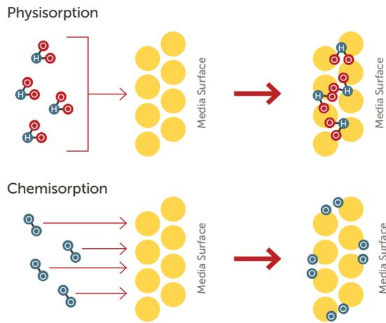
Figure 3: Comparison of how physisorption and chemisorption are used to remove common contaminants from the gas stream to prevent wafer defects.
