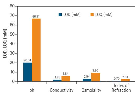
Figure 6: Limit of detection (LOD) and limit of quantification (LOQ) for pH, conductivity, index of refraction, and osmolality concentration measurements.<sup>9</sup>
