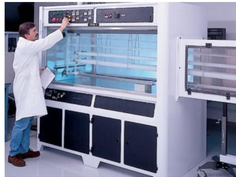
*This steam chamber – located in Entegris' Product Test Laboratory – is used to prequalify products for SIP conditions.*
