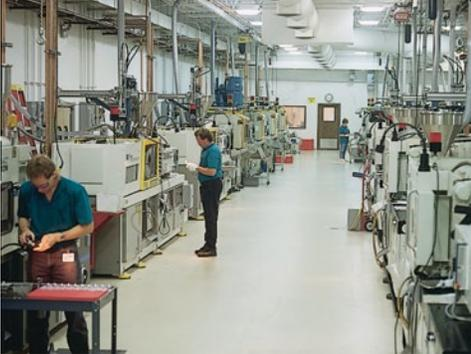
*Through product sampling and the use of statistical process control (SPC) tools, Entegris documents process parameters to ensure consistent, high-quality, injection molded products.*
