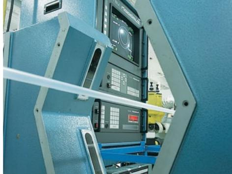
*An on-line laser measuring system continuously monitors the extrusion OD dimensions – ensuring dimensional specifications are met.*
