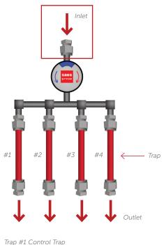
Trap #1 Control Trap Trap #2 Acids Trap #3 Bases Trap #4 Hydrocarbons/Refractory Compounds
