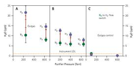
Pressure dependence of outgassing levels for three representative purifiers under  $N_2$  to  $H_2$  gas flow switch. Purifier C outlet moisture levels are maintained below instrument LDL (1 ppb) in the 100–600 Torr range.
