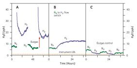
Comparison of moisture outgassing under sub-atmospheric conditions for three purifier technologies, A, B and C (HX media).
