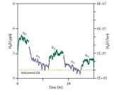
Measurement of HX purifier outlet moisture under dry (<50 ppb) inlet moisture during N<sub>2</sub>-H<sub>2</sub> flow switch.
