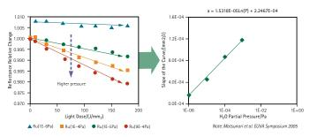
Reflectance loss dependence data of Matsunari et al. on  $H_2O$  pressure for Ru-capped Ru/Si optics under EUV exposure.
