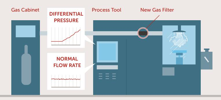
The system senses that the gas flow rate has been maintained and no risk exists. However, as pressure increases and gas velocity increases through the remaining open pores, the risk of particle liftoff increases. These particles may pass to the wafer and could be carried through further process steps, leading to wafer defects that weaken device performance.
