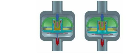
Figure 1. Gas Figure 2. Section view of the SPR. Left image flowing, right image no flow. stick assembly
