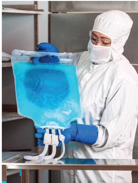
*Entegris' Aramus fluid-handling system is used to produce vaccines and is an example of the technology the semiconductor assemblies company is applying to life sciences. (Entegris)*
