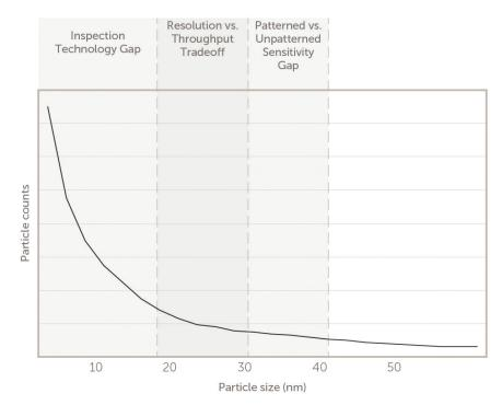
**Figure 2.** The defectivity power law, showcasing the relationship between the size and number of particles [6].
