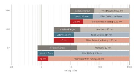
**Figure 4.** A comparison of the ability to detect particles, the size of killer and latent defects, and liquid filtration retention ratings typically used at 90 nm, 28 nm, and 7 nm nodes.
