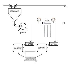
Figure 2. Filter test stand
