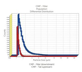
*Figure 3. CMP Slurry upstream/downstream of filter*
