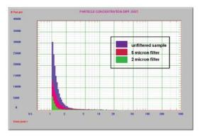
Figure 4. Inkjet ink unfiltered and filtered at 5 and 2 µm
