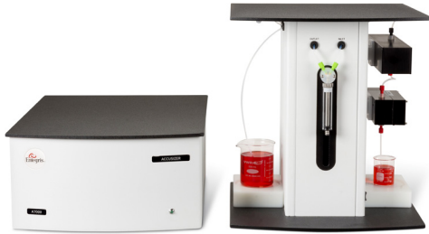
Figure 3. The AccuSizer SPOS system with SIS sampler.
