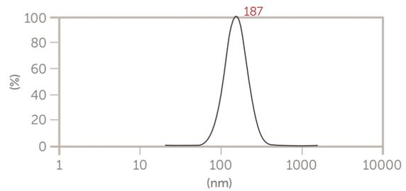
Figure 5. Liposome size after extrusion through 0.4  $\mu\text{m}$  membrane three times.
