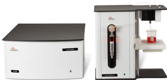
Figure 4. AccuSizer SIS liquid particle counter.
