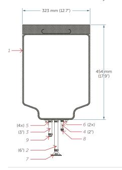
In designing the bag assembly, components were selected per the customer's requirements for integration into their process while special care was taken to ensure the materials would support the autoclave process. Silicone tubing with Oetiker retainment along with PVDF plugs and sanitary connectors were recommended.
