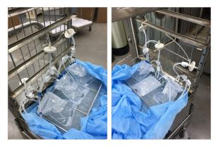
In the initial feasibility assessment, high success was seen at the smaller bag size (500 mL) and fluid volumes but not at the larger size (5 L) and volumes. We believe this was due to a not fully optimized autoclave cycle because only one parameter was changed from the standard liquid cycles used with rigid containers. The success of the smaller sizes was an indication that the Aramus bags can perform in this application with the proper steam sterilization cycle.
