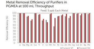
Total Metal Removal of Purifiers in PGMEA Feed: 5 ppb Each Metal
