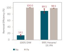
Figure 4. Metal removal efficiency of Purasol SN and SP with high metal loading in DI and 99% Hexane.
