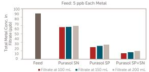
*Figure 2. Multi-metal removal efficiency of Purasol SP and SN in OK73 thinner.*
