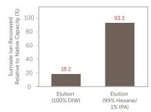
*Figure 5. Percent recovery of surrogate ion relative to native surrogate ion capacity for Purasol SN and SP with high metal loading in DIW and 99% Hexane.*
