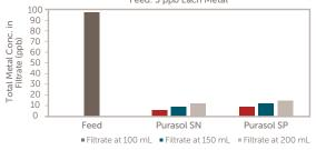
*Figure 1. Multi-metal removal efficiency of Purasol SP and SN in PGMEA solvent.*
