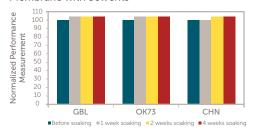
Figure 6. Effect of solvent exposure on the performance of Purasol SP and SN purifier membranes.
