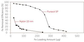
Figure 3. Profiles of Purasol SP and 10 nm Nylon membranes for 110 ppb Fe Challenge in OK73.
