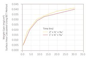
Oxidation resistance of SUPERSIC at 1200°C in an ambient air environment. The surface area was calculated using the BET method, which takes into account the surface area of individual grains.
