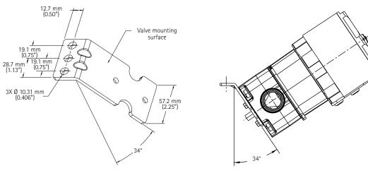
Optimum drain angle with valve sloped at 2% (1°)
