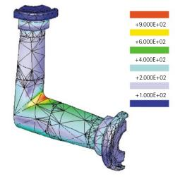
During component design, Entegris uses finite element analysis to identify high stress areas, and then adjusts the component design to minimize the stress affects.
