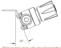
Optimum drain angle with valve sloped at 2% (1°)
