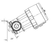
Optimum drain angle with valve sloped at 2% (1°)
