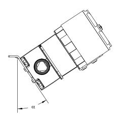
Optimum drain angle with valve sloped at 2% (1°)
