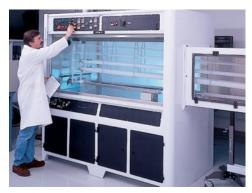
This steam chamber – located in Entegris' Product Test Laboratory – is used to prequalify products for SIP conditions.
