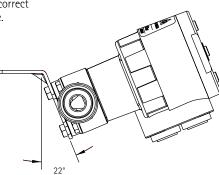
Optimum drain angle with valve sloped at 2% (1°)
