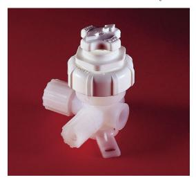
The valve used in this example is a ¼-turn manual right angle 2-way valve with a ¾" Flaretek port connection on the inlet and a ½" Flaretek port connection on the outlet.
