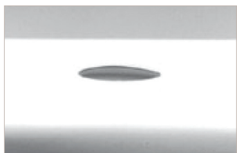
Aqueous chemicals instantly wet Rinsegard hydrophilic UPE membrane
