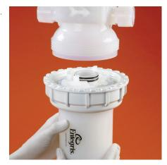
5. Adjust the torque setting to 45 N•m if using an E-FKM o-ring. For other o-ring types, 28.5 N•m.
