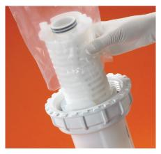
3. Using the end of the bag, the two finger tabs on the key can be used to turn the cartridge 1/4 turn; then lock the cartridge in place.
