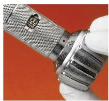
Once set, twist the lever at the end of the wrench clockwise to LOCK the setting in place.
