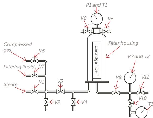
Figure 3. Steam-in-place system for liquid cartridge filters.
