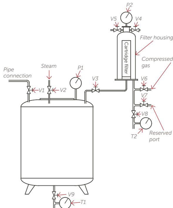
Figure 4. Steam-in-place system for vent filters.
