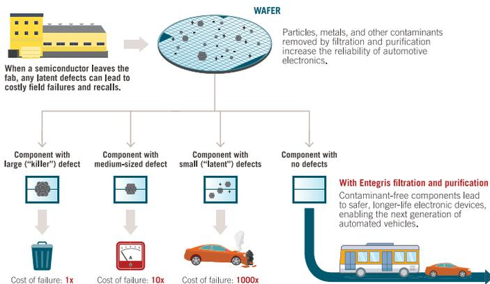
Figure 2. The cost of failure in automotive electronics.
