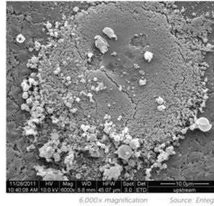
Figure 3. Various-sized particles captured in a chemical filter.
