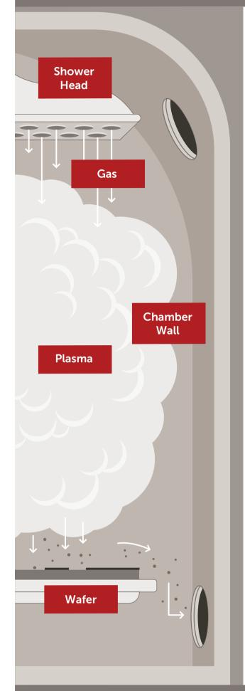
Traditionally, chamber parts and components in contact with wafers or chemicals were coated with metal oxides using plasma spray, anodization, and vacuum kinetic spraying.
