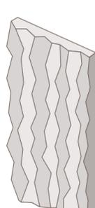
Temperatures >200°C yield rough, crystalline film in deposition.
