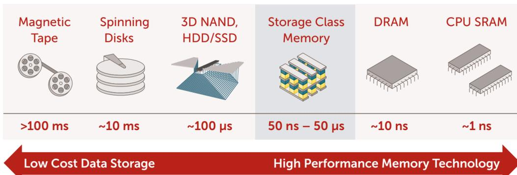
Storage Class Memory (SCM) occupies a critical middle ground, much more performant than non-volatile NAND flash memory, but not as costly or energy-dependent as volatile memory like DRAM or SRAM.
