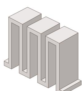
Vertical, high-aspect ratio structures require conformal deposition.
