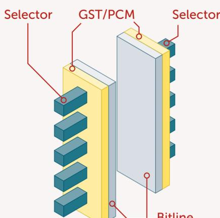
Arranging the PCM cell array vertically like 3D NAND may offer the most benefits in terms of density and lower cost of ownership.
