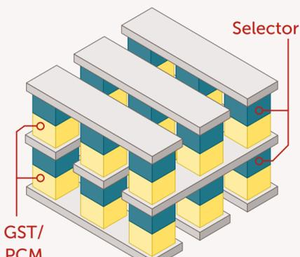
3D-stacked cross-point architecture is performant, but it must be built layer by layer and may not be cost-effective as it scales.
