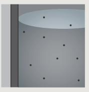
from the PE resin, improper process conditions, inadequately clean blow air used to make the container
