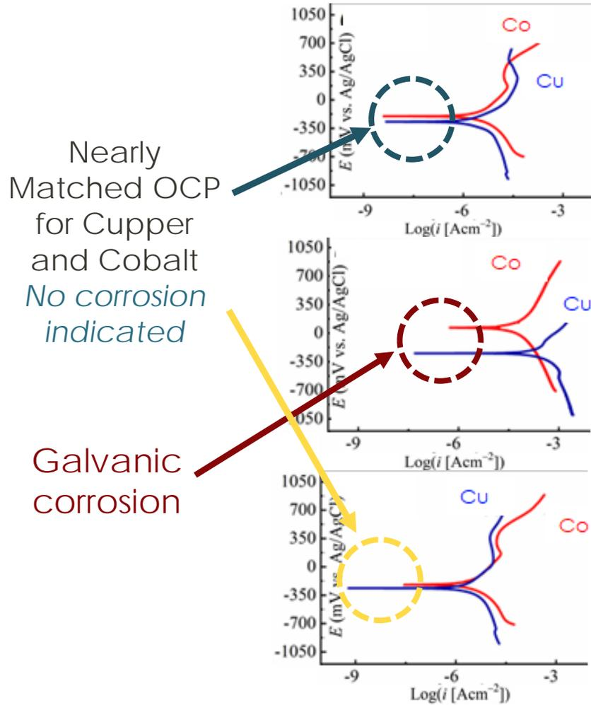
Data indicates the kinetics of the inhibitor reacting with cobalt is critical
