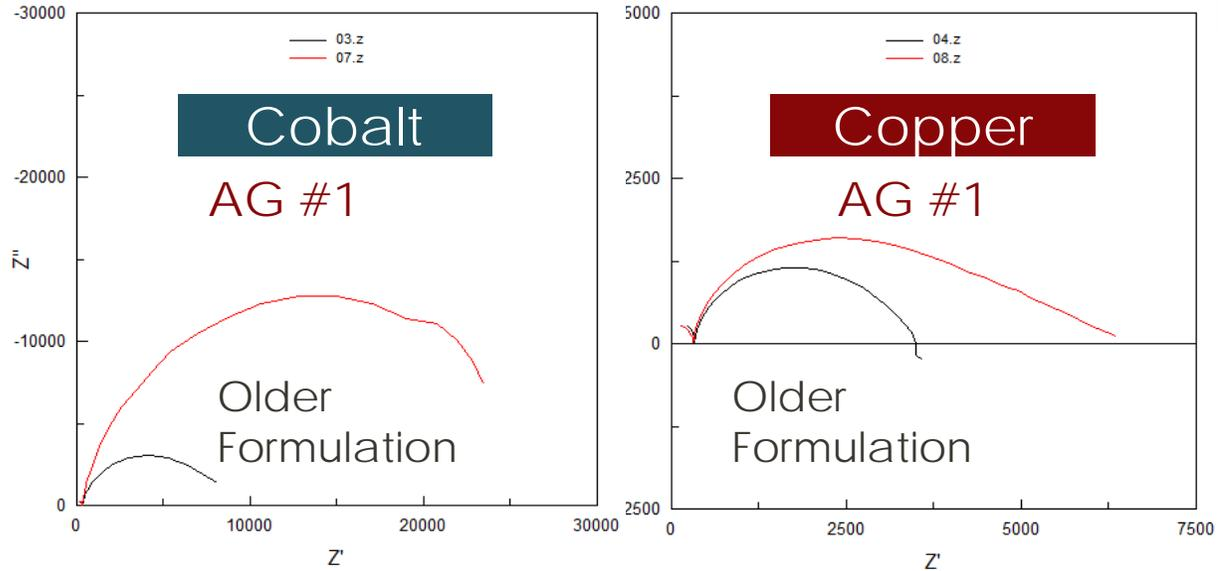
Higher impedance storage and loss components
