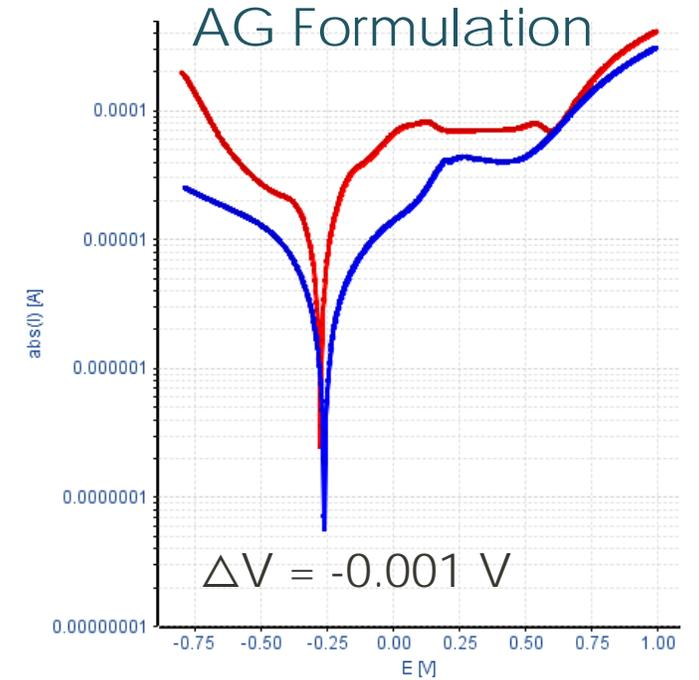
Nearly zero galvanic corrosion
