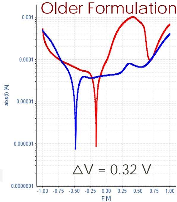
Anodic Co corrosion
