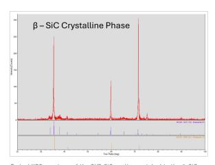
Typical XRD spectrum of the CVD SiC coating matched to the  $\beta$ -SiC or the 3C SiC phase from the library. The polycrystalline SiC has (111) and (311) dominant peaks, with the absence of any secondary peaks that can be attributed to the  $\alpha$  phase.
