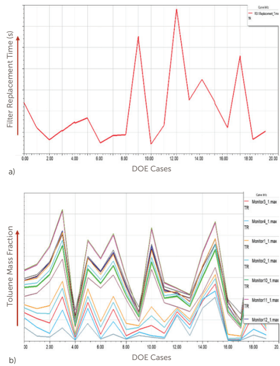
Figure 9. Filter replacement time (a) and virtual sensor prediction (b).
