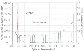
Figure 2. Water vapor and oxygen trend vs. cylinder pressure.
