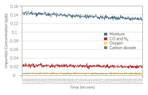
Figure 8. Impurities concentration at the outlet of a palladium purifier.
