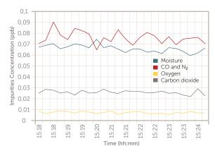
*Figure 5. Typical impurities concentration at the outlet of a getter purifier.*
