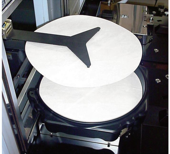
*Entegris multilayer nonwoven inserts are transferred into a 300 mm SmartStack horizontal wafer shipper by an automated tool.*
