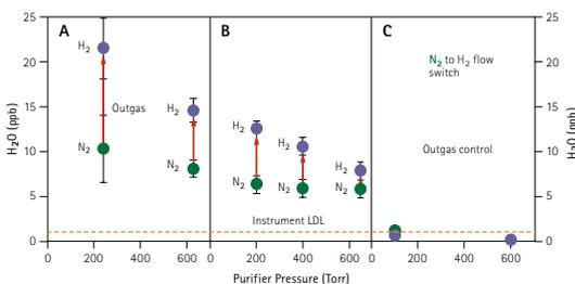
Pressure dependence of outgassing levels for three representative purifiers under  $N_2$  to  $H_2$  gas flow switch. Purifier C outlet moisture levels are maintained below instrument LDL (1 ppb) in the 100–600 Torr range
