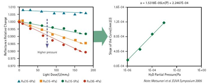
Reflectance loss dependence data of Matsunari et al. on  $H_2O$  pressure for Ru-capped Ru/Si optics under EUV exposure.
