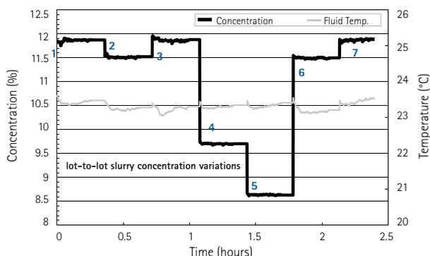
Variation from batch to batch is easily noticeable, nearly a 3.5% range. Five of the samples monitored were roughly the same concentration percentage, but even small differences can lead to product yield defects. Customers often require monitoring capabilities into the hundredths place. We quote our NX-148 product down to a 0.01 wt% resolution. With incoming chemical variations of this magnitude the NX-148 product will have no problem detecting and signaling an engineer.
