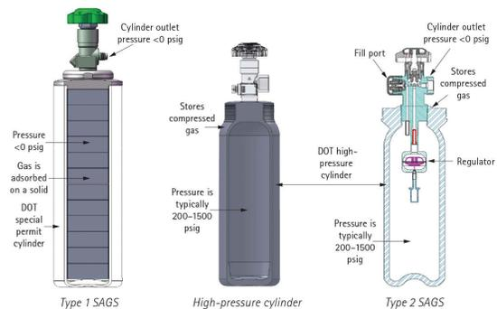
Fig. 4. SAGS systems as compared to the traditional high-pressure cylinder.
