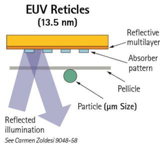
Figure 1. Illustration of an EUV pellicle for reticles.
