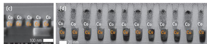
Figure 3(a) shows the SEM top view of the test structure before Co selective deposition. The test structure went through a wet surface preparation clean first, then Co selective deposition was carried out at 250°C. Figure 3(b) is the SEM top view of the structure after Co deposition. There was no Co growth observed on the ULK surface. Figure 3(c) is the cross-sectional view of the via structure filled with Co. No voids were observed because the Co growth is selective and bottom-up.
