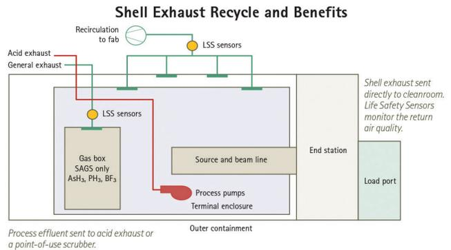
Fig. 3. New design configuration for shell exhaust recycle.
