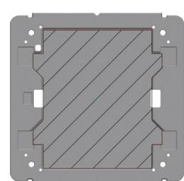
Figure 4. An overlay of the pellicle pocket requirement (shaded area) and the pellicle pocket of the Entegris pellicle-compatible EIP baseplate.
